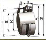
Stationary based, unitised elastomer bellows seals, utilised in small shaft diameter applications. Compact, unitised design, provides excellent flexibility in accommodating shaft mis-alignment and with quality seal face materials, to extend seal performance and life. The adequate shaft clearance enables one size to be used on a number of shaft sizes, whilst being stationary based increases the seals bi-directional rotational speed capabilities.
